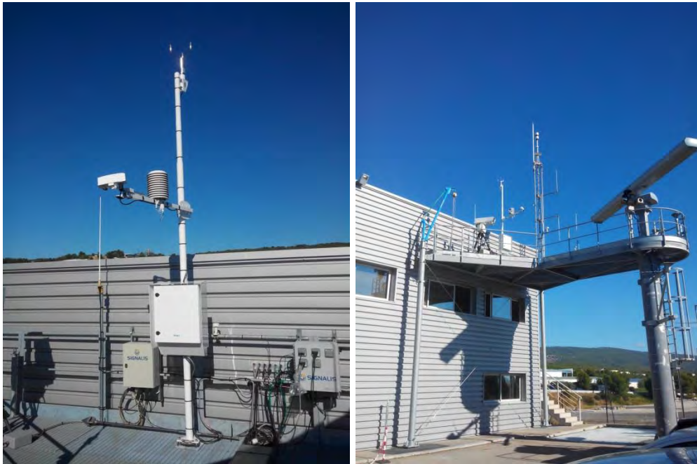
Image: Vaisala sensors and Automatic Weather Station (AWS340) installed at SIGNALIS R&D Platform – La Ciotat (South of France)
